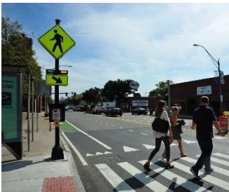
Rectangular Rapid Flashing Beacon (RRFB)
